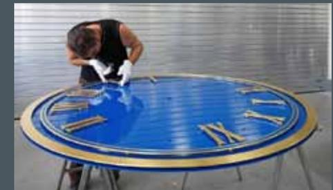
*in our metalworking shop. For cutting production and gearing we use the latest CNC machines. Our newly accomplished painting centre is likewise modern, innovative and energy-saving. The heart of this painting centre is a 9 m long, 4.50 m wide and nearly 3 m high combined painting and drying system, in which all the dials, hands, tower decorations and numbers are coated and lacquered and the gilding work is carried out. Energy production in our works relies mostly on geothermal energy.*
